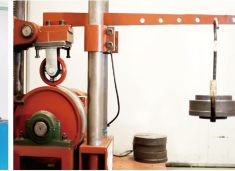
Load Test For Heavy Duty Casters 重型脚轮载重行走测验
